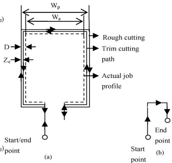
Figure 2 Wire paths planning for machining of test specimen in trim cutting followed by rough cutting
